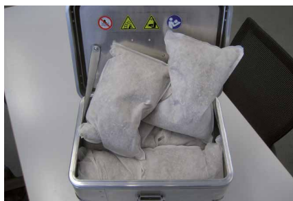
Thermal insulation material, e.g. Vermiculite
